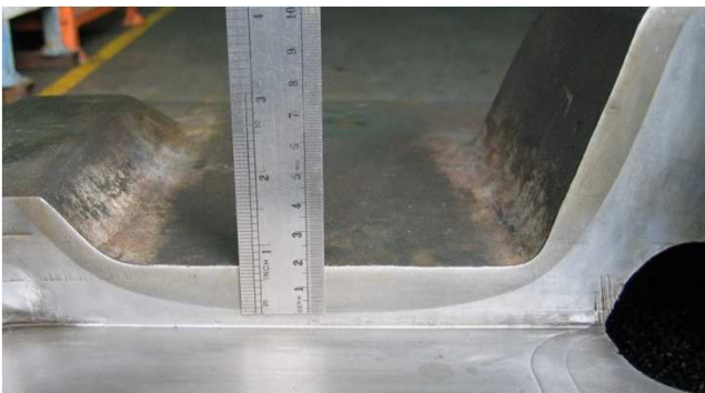
Running surface case depth 17.5 mm
