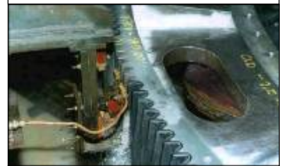
Computerised full contour induction hardening of large Slew Gears and Bearing Race Ways
