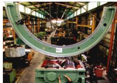
SELF ALIGNING, TWIN PINION MILL DRIVE GEARBOX
